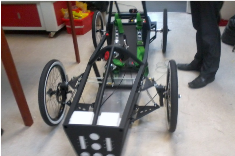
First, we had to assemble the Greenpower kit car. This involved adding the wheels, steering and drive system.
