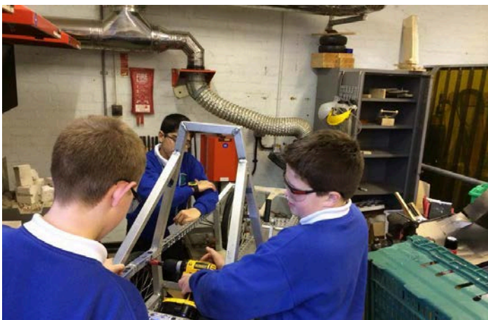
Once the rolling chassis was complete, it was time to drill more holes! This was all to save weight.
