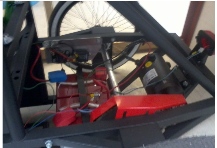
We then wired all of the electronics into the car, and put in the tray for the batteries.
