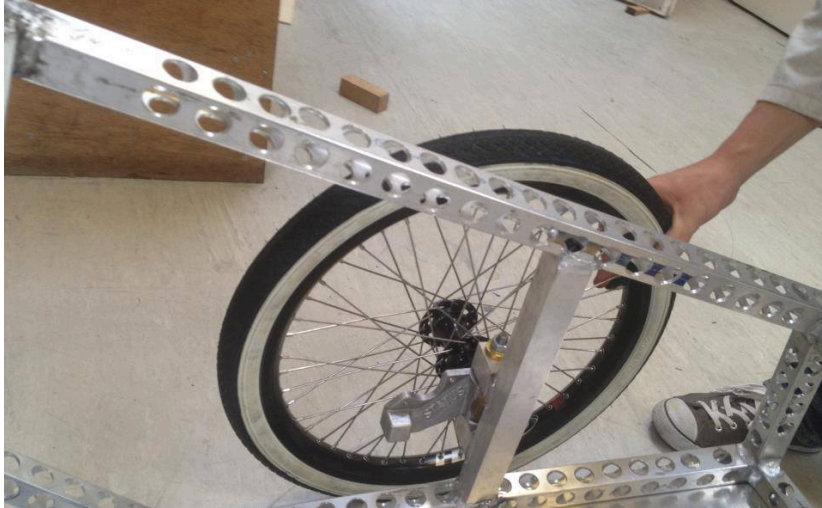
The wheels are then attached to the chassis, and adjusted to remove any camber.
