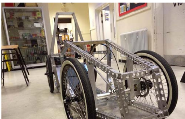
The steering is then added. This involved machining a piece of steel bar for the connection to the wheel and adding the rose joints to the steering arms.
