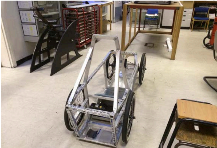
We then added the battery tray at the back of the car and mounted our motor!
