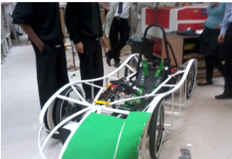
Next, a shell was created over the chassis by bending pieces of plastic to create the shell shape.
